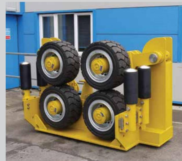
A 3 tonne adjustable hydraulic cable tensioner
